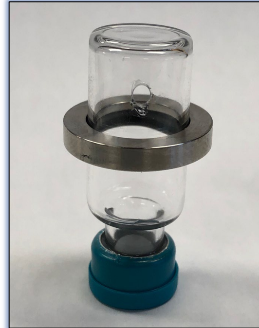
Sample Fixture set-up. Note drilled hole in vial sidewall
