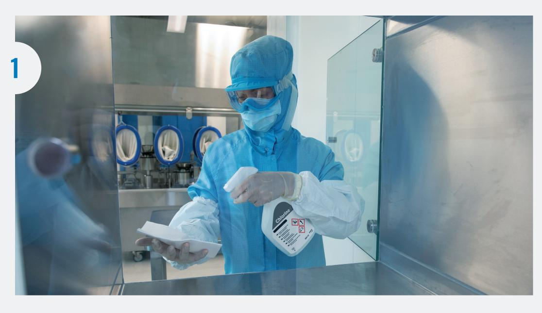
Manual disinfection of containers carries a higher risk of introducing contamination into an isolator due to IPA lacking sporicidal activity but is typically quicker than an automated bio-decontamination process and avoids the risk of damaging living materials.
