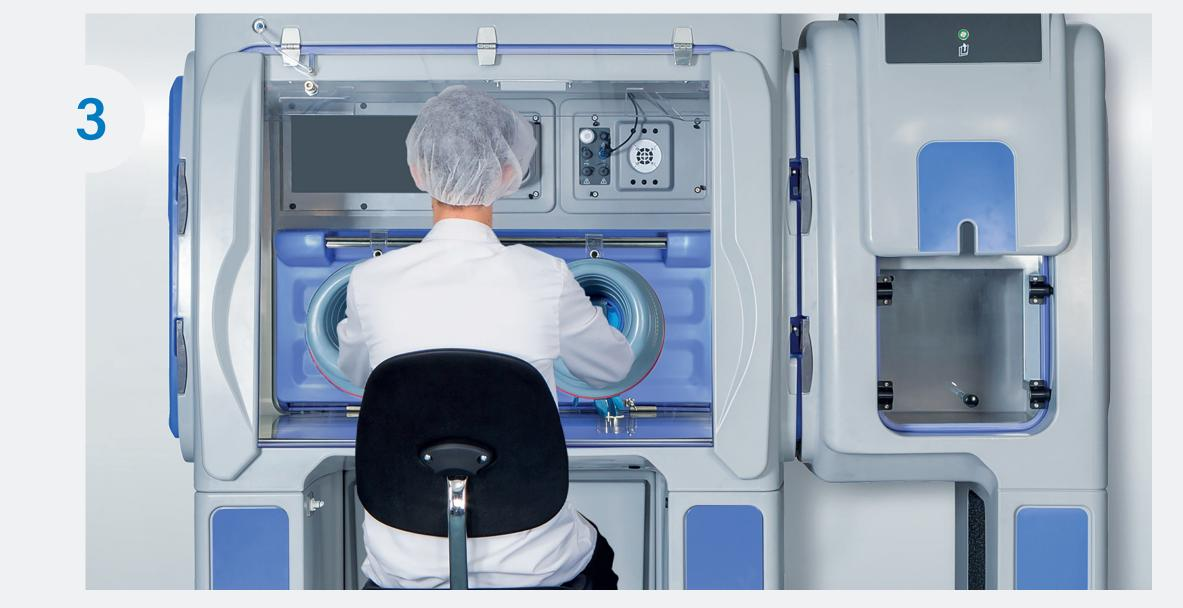
The **automated bio-decontamination** solution is the most robust method for contamination control but may not be possible. Ingress testing should be conducted to determine whether the container is compatible with hydrogen peroxide vapor bio-decontamination.
