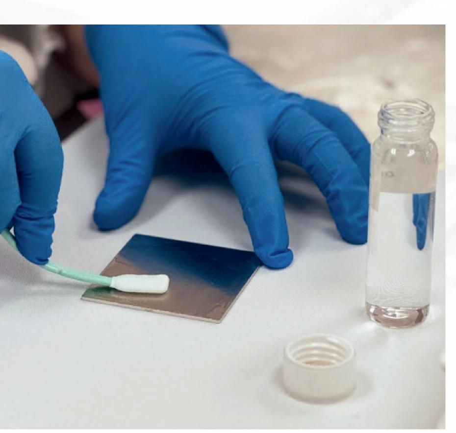
Figure 2. Hand swab sampling during recovery study at Hyde Analytical Laboratory
