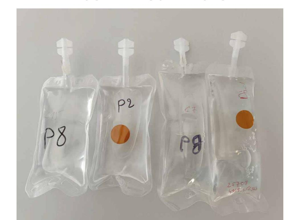
From left to right: 200ml capillary PC, 200ml laser drilled disk PC, 300ml capillary PC, 300ml laser drilled disk PC
