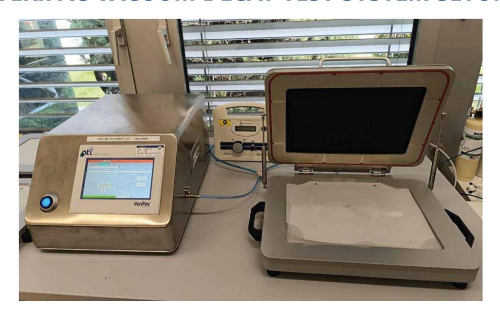
Test setup with VeriPac, Test Chamber and Microcallibrator
