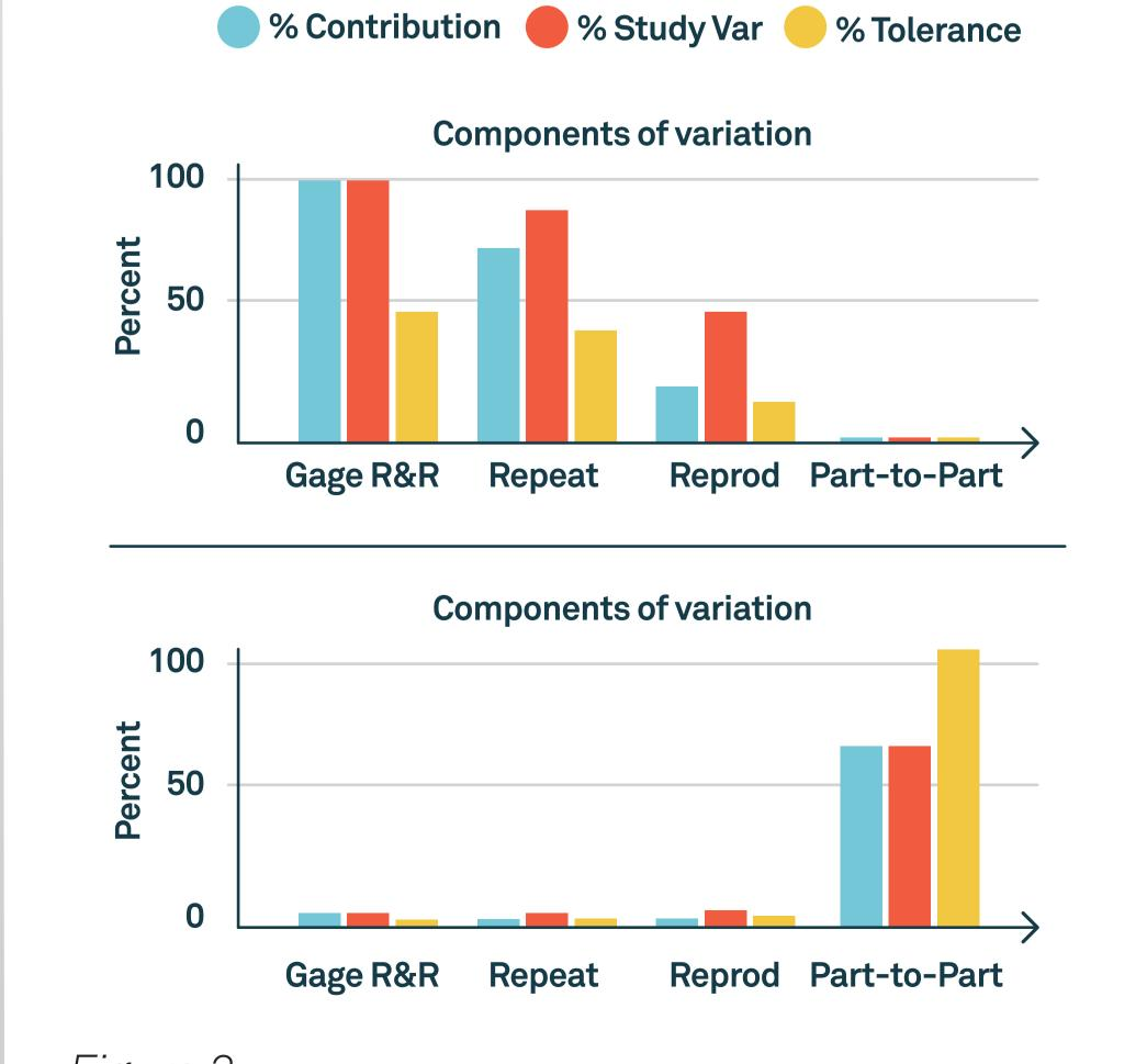
Figure 3 Gage R&R analysis-destructive (top) or surrogate (bottom)
