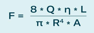
Hagen-Poiseuille equation – giving a very first indication but does not replace realistic test conditions Formula valid for Newtonian fluids with F – frictionless travel force; Q – volumetric flow rate;
