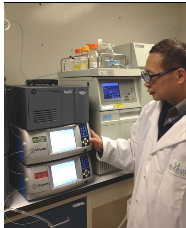
Analytical chemist operating Multi-Angle Laser Light Scattering (MALLS)
