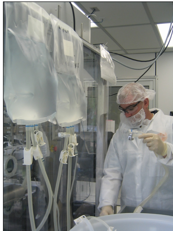
Attaching buffers to chromatography skid
