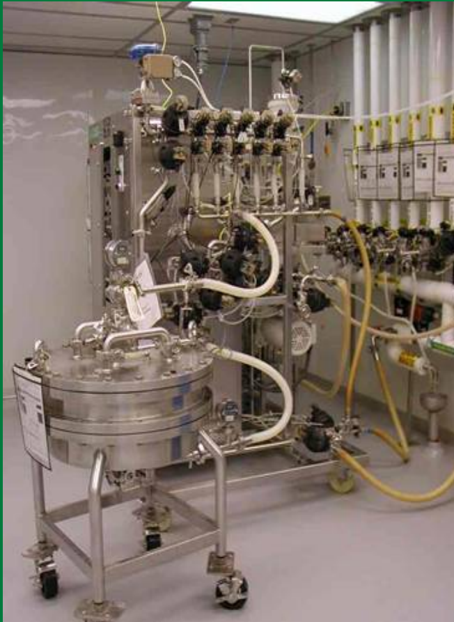
60 cm Chromatography Column, Skid, and Piping
